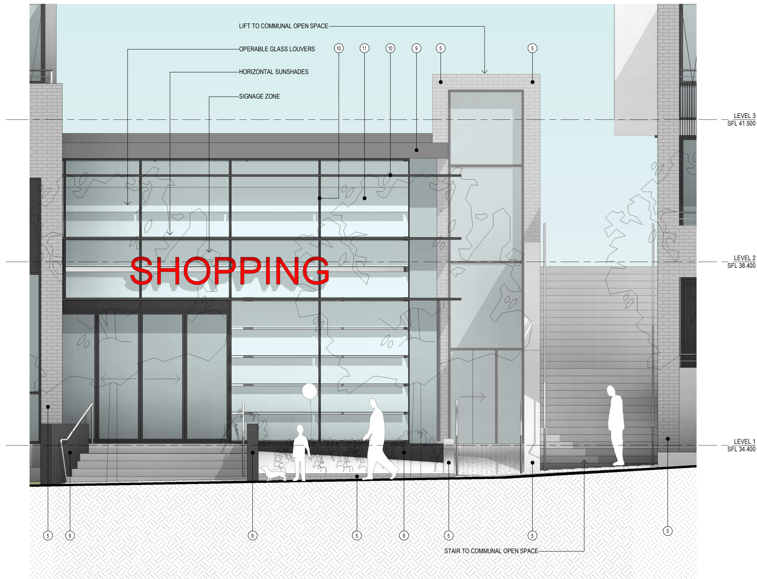
2 ELEVATION - NSR-3 ENTRY 1:50
